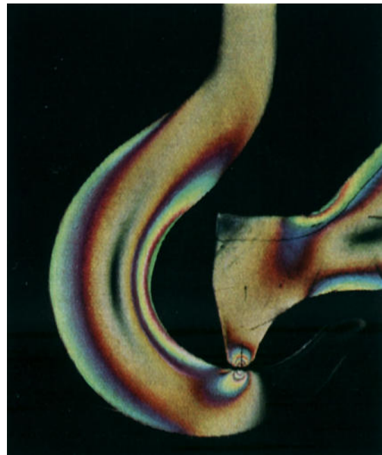
Loaded hook in circularly polarized white light
